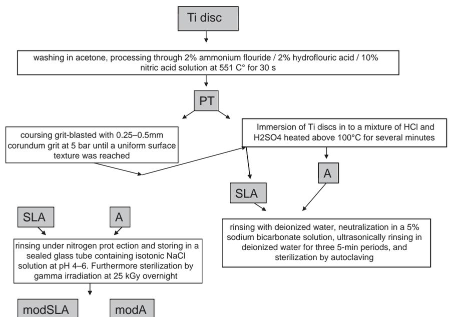
**Fig. 1.** Fabrication of pre-treated (PT), acid-etched (A), large grit-sandblasted acid-etched (SLA) as well as acid-etched, hydrophilic (modA) and large grit-sandblasted acid-etched, hydrophilic (modSLA) titanium surfaces.
